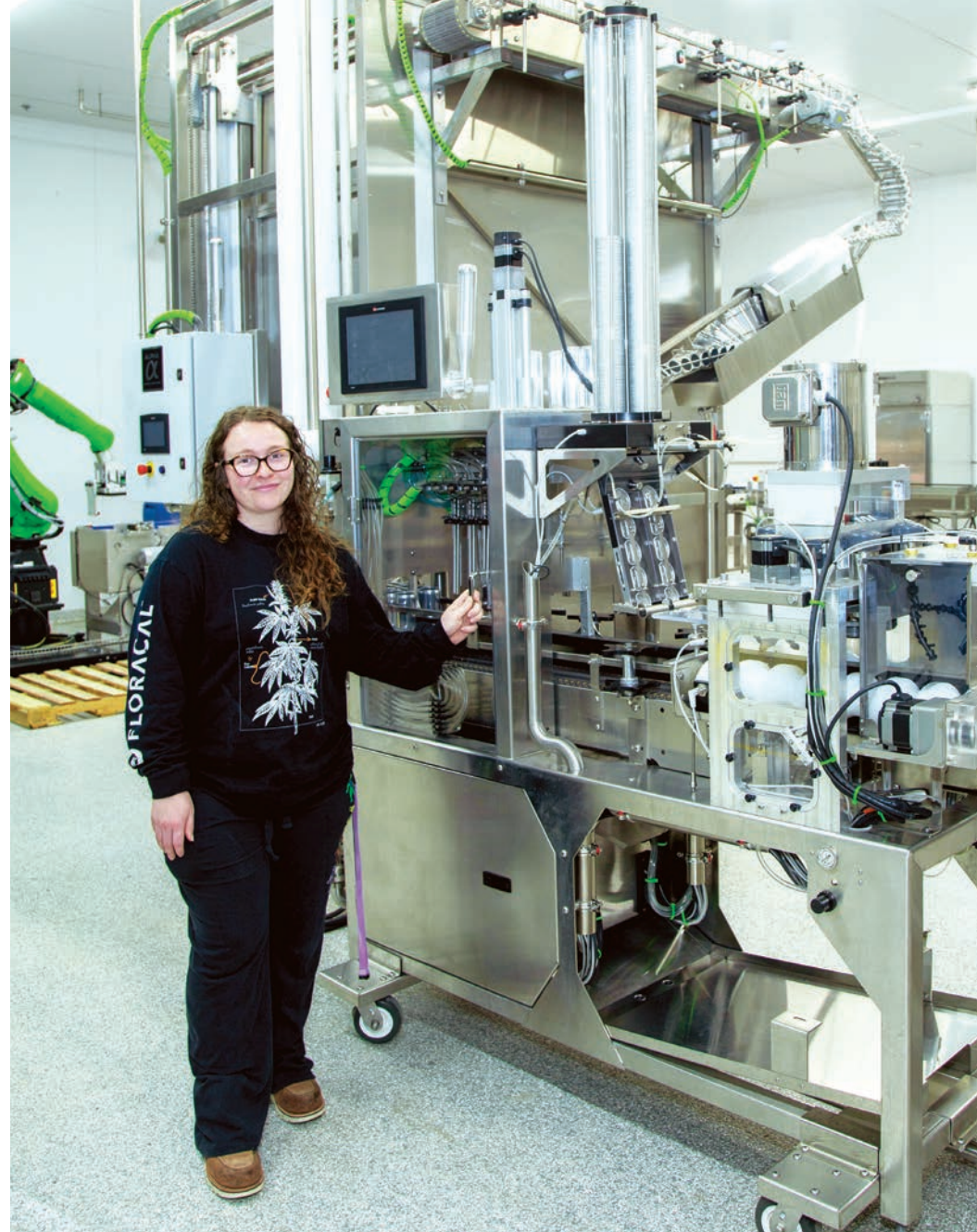
Gabrielle Isaacks, operations coordinator for CoPack Industries, shows off the Alpha Brewing-brand equipment that will feed cans from pallets at the top of the machine into a “filling station” where the cans will be filled with THC-infused beverages and then seamed and sealed. PHOTO BY STEVE HINRICHS.
