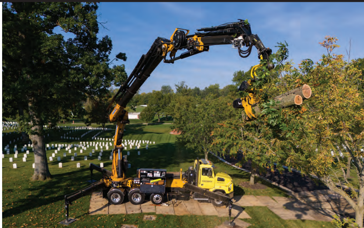
Jake Erdman with OakBros Trees uses their knuckle boom crane to move logs from a large removal to a collection point. PHOTO COURTESY OF THE BETTER CONTRACTOR
